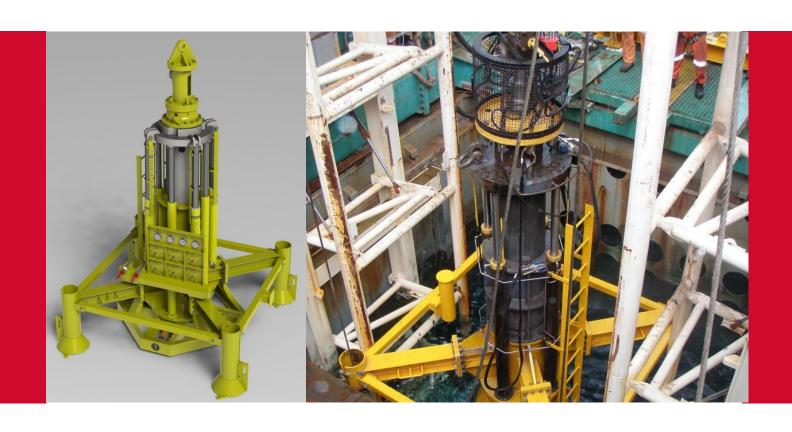
An ITC and/or Tubing Hanger Running Tool (THRT) is adapted to the SSTD. The SSTD is run onto the well/subsea tree using a deck crane or deck winch and the hydraulic umbilical. The tool is then locked to the subsea tree, the THRT is engaged and locked to the ITC or TH. The ITC or TH is then disengaged from the tree by activating the jacking system of the SSTD. The SSTD is now recovered to surface with the UTC or TH connected to the SSTD.
